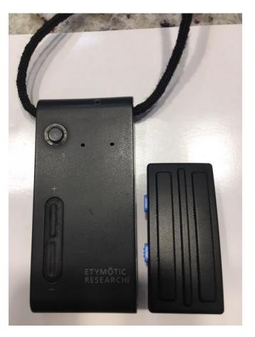
staying together. The range of the between the receiver and transmitter unit appear to be about 30 feet. The units do not have to be in the line of sight for them to work with each other. The one concern I have is that in transmitter mode, you have to be careful how they are positioned--- the microphones do not appear to be omnidirectional. If the speaker turns away from the microphone, speech may not sound as clear.
